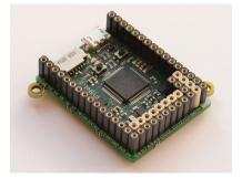
MicroPython is an efficient implementation of the programming language Python 3 with the standard libraries and is optimized to run on embedded hardware, specifically for the Pyboard. It also contains hardware-specific modules to make use of different low-level hardware, for example: I2C and GPIO.
